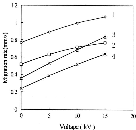
**Figure 7.** Effect of voltage on retention. Column: EP-150-25-5-SCX mobile phase 70% acetonitrile in 5 mM  $\text{KH}_2\text{PO}_4$  buffer pH 4.5; pressure: 500 psi; voltage: 0, 5, 10, 15 kV; sample: 1 indapamide, 2 thiourea, 3 atenolol, 4 isoprenaline.
