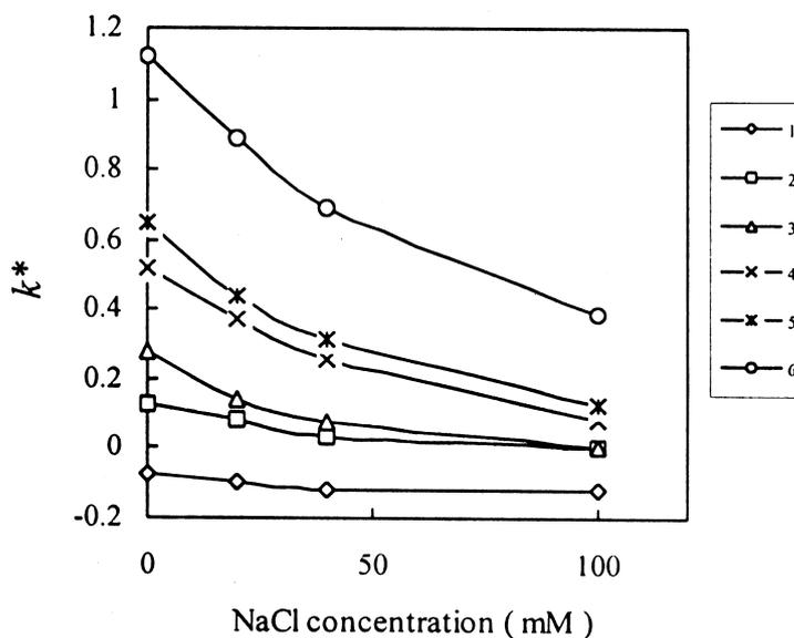
**Figure 4.** Effect of ionic strength on pCEC separation. Column: EP-100-25-5-SCX mobile phase vary concentration NaCl in 5 mM  $\text{KH}_2\text{PO}_4$  buffer pH 4.5 which consists of 70% acetonitrile; pressure: 500 psi; voltage: 5 kV; samples: as in Fig. 2.
