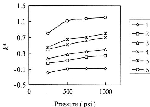
**Figure 6.** Effect of pressure on retention. Column: EP-100-25-5-SCX mobile phase 70% acetonitrile in 5 mM KH<sub>2</sub>PO<sub>4</sub> buffer (pH 4.5); voltage: 5 kV; samples: as in Fig. 2.
