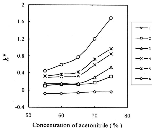
**Figure 3.** Effect of concentration of acetonitrile on retention. Column: EP-100-25-5-SCX mobile phase vary concentration acetonitrile in 5 mM  $\text{KH}_2\text{PO}_4$  buffer pH 3.5; pressure: 500 psi; voltage: 5 kV; samples: as in Fig. 2.
