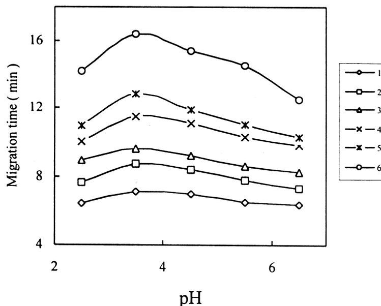
**Figure 5.** Effect of pH on retention of pCEC separation. Column: EP-100-25-5-SCX mobile phase 70% acetonitrile in 5 mM  $\text{KH}_2\text{PO}_4$  vary concentration pH value buffer; pressure: 500 psi; voltage: 5 kV; samples: as in Fig. 2.
